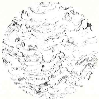
Spraying material : SUS 410 (13% Cr stainless steel)(200 magnifications)
